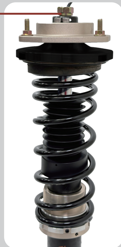
OEM top nut (M14, with 70Nm of torque)
